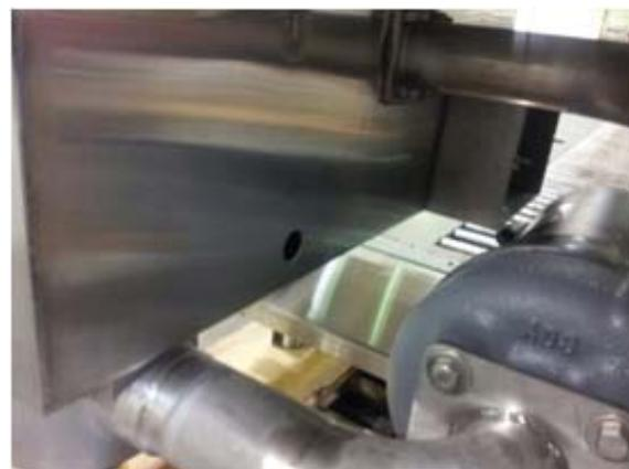
Showing 7/8" detergent probe hole behind pump motor
