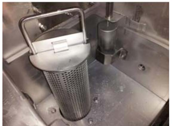
Pump filter in drain sump
