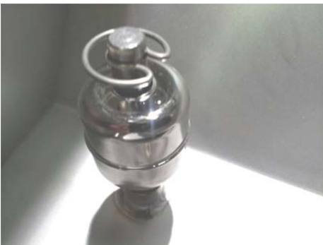
Control float, "O" mark should be on top
