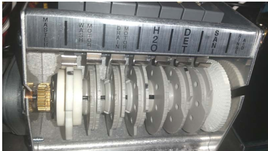
ASQ cam timer, fixed cams are MASTER, WASH MOTOR and DRAIN MOTOR
