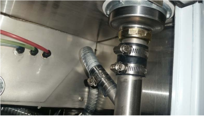
Drain hose connection to drain pipe
