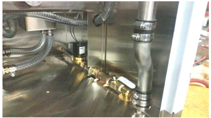
Showing 1/2" H2O solenoid, also stainless 1.5" drain tube
