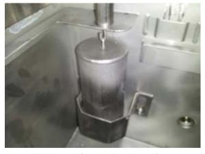
Wash tank float and tank overflow
