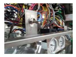
De-lime switch in HT25 control box
