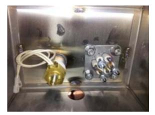
Showing thermostat and sustainer heater terminals\*
