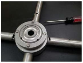
Remove 4 screws and lift top shell
