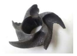
Impeller damaged from high acid solution
