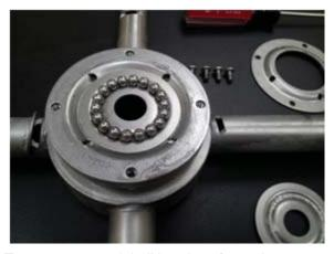
Top race removed, ball bearings for replacement
