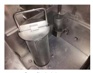
Pump filter in drain sump
