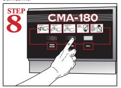
Press "AUTO FILL" immediately after power is turned on. Timer will automatically fill until the water overflows into the scrap trap.
