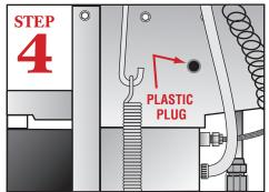
Remove the plastic plug to install the detergent fitting (provided by your dispenser supplier; CMA does not supply).
