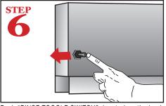
Push "RINSE TOGGLE SWITCH", located on the back of the control box, to fill the booster tank.
