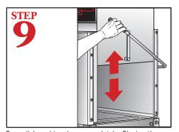
Open dishmachine doors completely. Closing the doors will automatically activate the machine.
