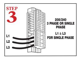
**3 Phase:** Connect power supply wires, L1, L2 and L3 to the appropriate terminals marked L1, L2 and L3 on the power block. **Important:** If one of the three wires has higher voltage it must be inserted as L-2.
