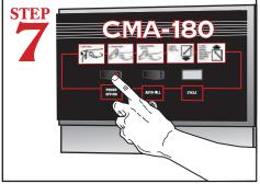
Press "POWER ON/OFF" rocker switch to turn on dishmachine.
