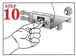
Adjust the temperature by removing the panel in front of the respective heater and turning the adjustment post. Wash temp. 155°F. Rinse temp.180°F.
