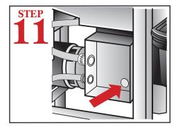
Remove the stainless steel plug to install the detergent probe (provided by your dispenser supplier; CMA does not supply).
