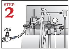
Connect dishmachine to hot water source-minimum 140°F if unit is equipped with a booster heater. If 140°F is not available, order a 2 minute time cycle (120°F minimum temperature required). A minimum of 180°F is required if unit is not equipped with a booster heater.
