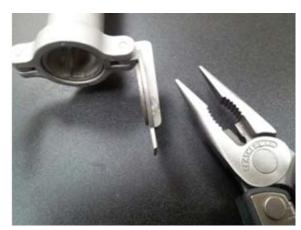
Straighten tab in line with the coin edge to tighten latch
