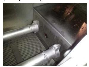
Showing hole at the side of tank, 7/8" detergent fitting
