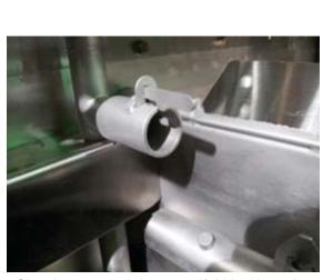
Showing pumped rinse manifold locking tab
