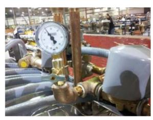
Final rinse manifold with pressure gauge, 20 psi flow req.
