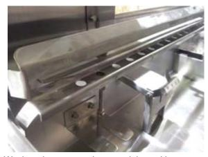
Wash tank sequence bar, pendulum with magnet
