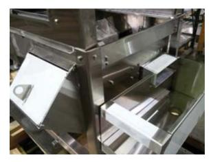
ADC-66 power scrapper, overflow to scrap box
