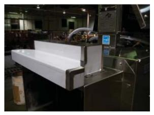
Vent attachments to end shield, 4" x 16" opening
