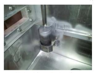
Wash tank float and tank overflow
