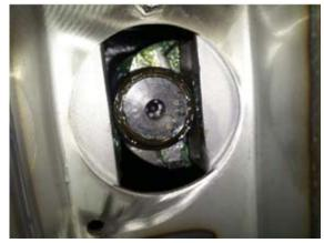
Cam bearing screws into cam block B
