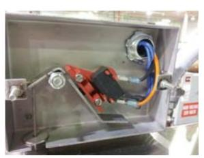
Showing "float" switch that controls fill water & heater
