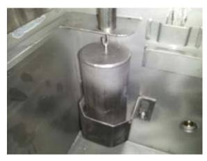
Wash tank float and tank overflow
