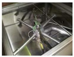
Final rinse arm twisted into transfer tube
