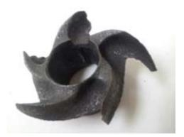
Impeller damaged from high acid solution
