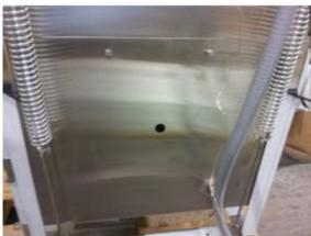
Showing back of tank, 7/8" detergent bulkhead fitting hole
