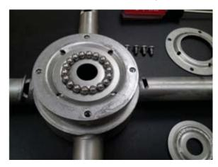
Top race removed, ball bearings for replacement
