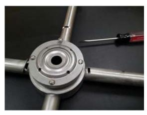
Remove 4 screws and lift top shell
