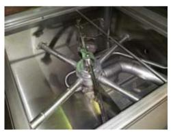
Final rinse arm twisted into transfer tube
