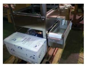
Showing PRV, ASSE approved air-gap, final rinse gauge
