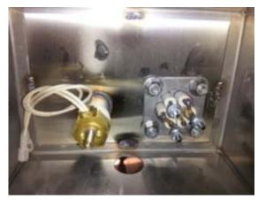
Showing thermostat and sustainer heater terminals\*
