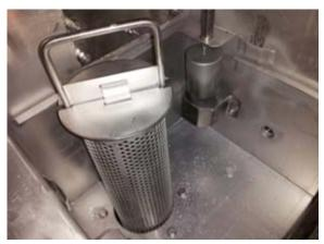
Pump filter in drain sump
