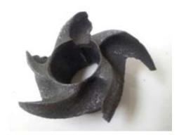
Impeller damaged from high acid solution
