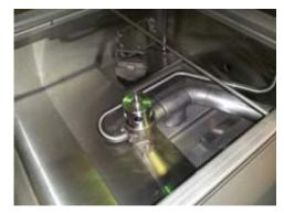
Showing spray arm base & transfer tube Wash arm w/bearing installed on base
