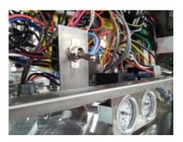
De-lime switch in HT25 control box
