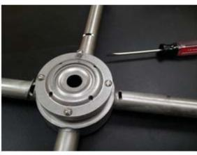
Remove 4 screws and lift top shell
