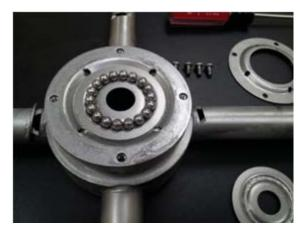
Top race removed, ball bearings for replacement
