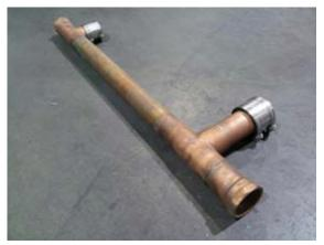
HT-25 drain manifold with "no-hub" connectors
